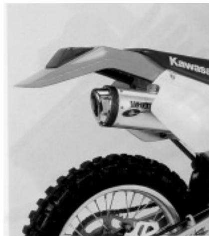
By adding E-Series Discs, you are increasing the outlet area and thereby increasing: the powerband for more top-end power, the sound level and leaning out the carburetion. By subtracting E-Series Discs, you are decreasing: the outlet area and thereby decreasing the powerband for more bottom end or torque, the sound level and enriching the carburetion.
